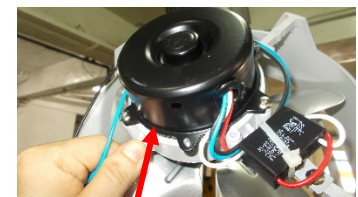
Drain hole of motor must face down. 馬達排水孔必須向下。
